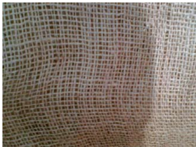
Fig. 4 : Open-weave light jute hessian fabric
