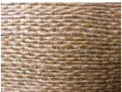
Fig. 18(c) : Jute-coir-synthetic blended fabric (Blending with coir increases the durability of the geotextiles. The structure of the fabric increases the anti-slip property.)
