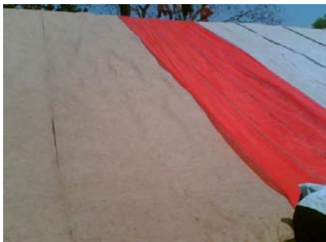
Fig. 5 : pp leno-weave fabric backed by jute nonwoven fabric
