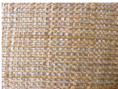
Fig. 18(a) : Plain weave fabric (HDPE in machine direction and jute- yarn in cross-direction)
